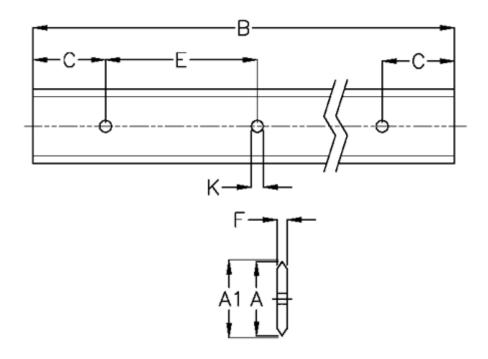
$\begin{array}{lll} A & = 76 \\ A1 & = 76.81 \\ B & = 266 \\ C & = 43.0 \\ E & = 90 \\ F & = 9.43 \\ For bearing = J54 \end{array}$
